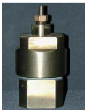
Figure 3: Pressure Vessel for PFOS Decomposition
